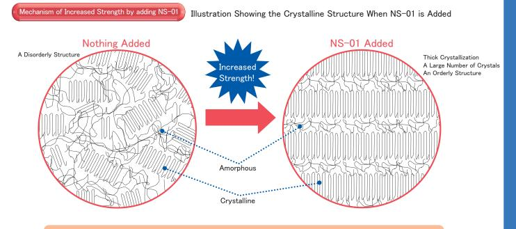
By promoting crystallization of the resin, an orderly structure is formed. Even with the increased crystallization, the transparency of the film does not change.
